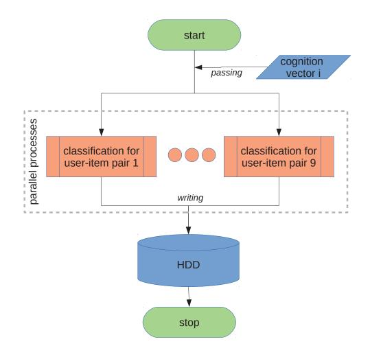
Figure 6.13: Flow chart representing the algorithm of processing and distributing data on a single HPC computing node
