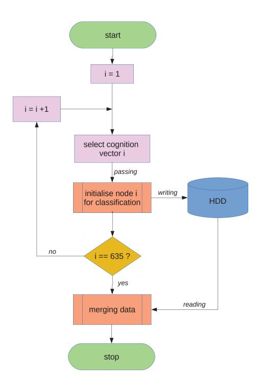
**Figure 6.12:** Flow chart representing the algorithm of splitting, distributing, and merging the data across the HPC
