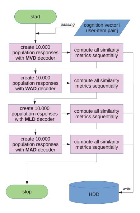
**Figure 6.14:** Flow chart representing the main classification algorithm performed by each parallel process on each node
